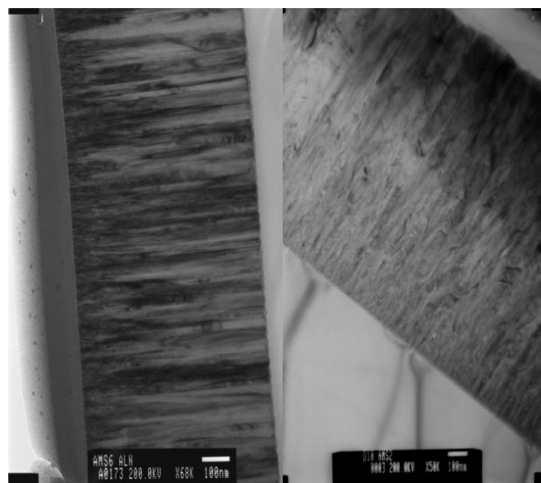
Figure 8. TEM micrographs of high (left) and low (right) quality AlN films.
